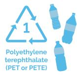
Properties: Clarity, barrier to gas and moisture, heat resistant, toughness.
